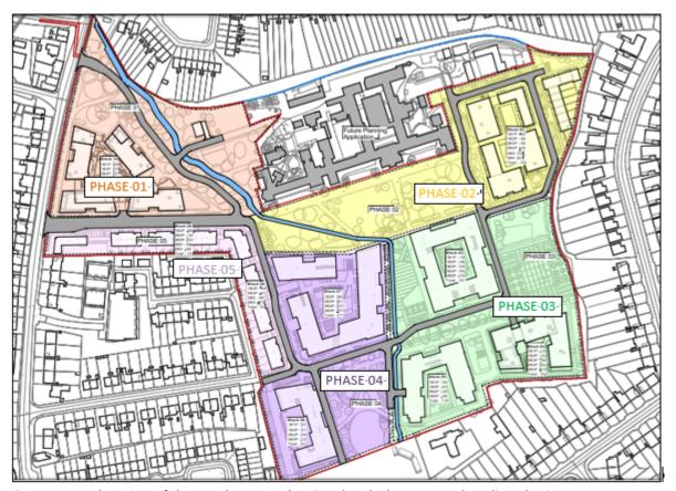
Figure 9.11 - Plan View of the Development Showing the Block Layout and Outline Phasing.
