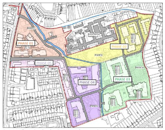
Figure 5.1: Illustrative Plan showing proposed construction phasing.
